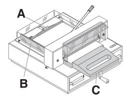
Position the paper on the backgauge (A) and the side lay (B). To move paper stacks, please use the paper knock-up block (C). Run backgauge to the front for turning the paper stack.
