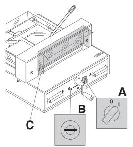
Position the main switch "I" ( $\bf A$ ) Insert the key the control system and move it to the right ( $\bf B$ ). Open the safety guard ( $\bf C$ ). The machine is now ready for use.
