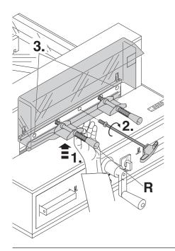
Push the blade changing tool to the top with your hand (1.). First, lightly tighten the middle blade screw with your other hand (2.) and then both blade screws left and right (3.). Remove the blade changing tool (R) (unscrew the grips).
