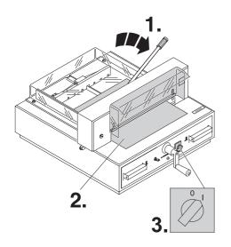
Open the clamp by moving the clamp lever to the right (1.). Remove all tools and distribute paper along the entire cutting length (2.). Turn main switch to position "I" (3.).
