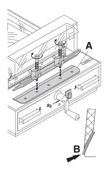
Take the exchange blade carefully out of the blade box and screw it to the blade changing tool (A)
