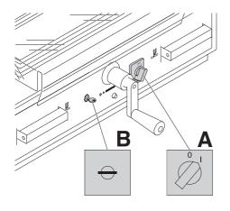
Main switch to position "I"? (A) Control system activated? (B) (Turn key to the right) Release a cut see page 18.
