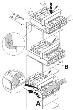
2 strong people are required to lift the machine onto the cabinet. Beware of fingers! Do not hold onto the actuators (B) when lifting the machine out of the packaging! The operating side of the machine must align with the cabinet (A)!
