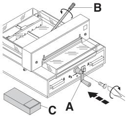
Screw on the backgauge crank (A). Screw on the handle (B) (only 4315) found in the tool set (C).
