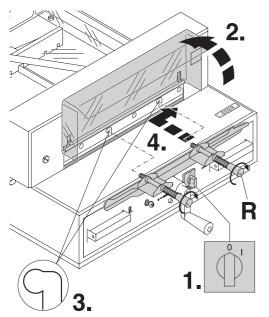
Position the main switch to "0" (1.) Open the safety guard (2.). Remove the 2 blade screws on the elongated holes (3.). Then put the blade changing tool (R) into place and fasten it to the blade (4.).
