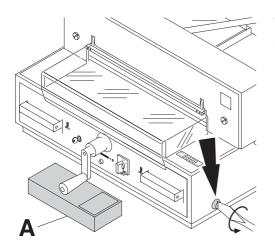
Turn the blade depth adjustment screw to the left until it stops (screwdriver found in tool set (A).
