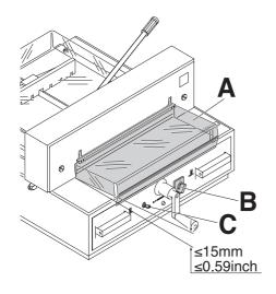
Before working with the machine and after every blade replacement the automatic cut-off function of safety guard (A),(correct if distance between cover and table is < 15 mm) main switch (B) and control panel (C) must be checked.
