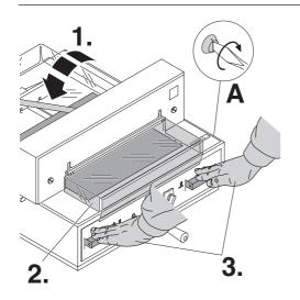
Close the clamp by moving the clamp lever to the left (1.) Close the safety guard (2.) Lower the blade by pressing both cutting buttons (3.) If the last sheet of paper is not completely cut, gradually turn the knob for blade-depth adjustment (A) ¼ turn to the right until the paper is cut along the entire length. (1 turn = 1.5 mm)
