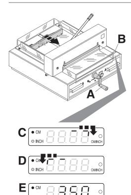
The measurement is set with the backgauge crank.(A) The symbol – rotary direction – ¬ moves to the right on the display (B) (see picture C). The rotary direction of the backgauge crank (A) is indicated on the right.
