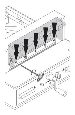
Tighten all 5 blade screws with a torque of 10Nm.
