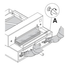
Paper cutting test. If the last sheet or several sheets are not completely cut, gradually turn the knob for blade depth adjustment (A) ¼ turn to the right until the paper is cut along the entire length. Do not set too low as blade will become blunt sooner.
