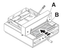
Optical cutting red line (**A**). Blade cuts on the front edge (**B**) of the light beam. (Only use when no exact cut is required).
