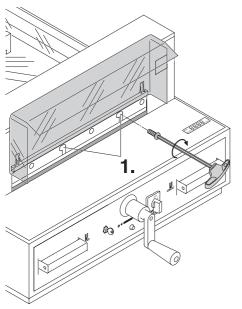
Lightly tighten the 2 blade screws on the elongated holes (1.).
