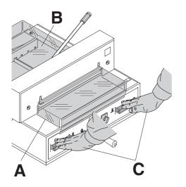
The dangerous cutting movement is safeguarded by a movable guard (A), rear screwed safety guard (B) and a safety two-handed control system! (C)
