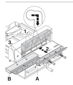
Remove the remaining 3 screws (1.). Push the blade and blade changing tool (A) to the right and lower to remove (2.) Place the blade into the blade carrier (B) and screw it into place (3.).
