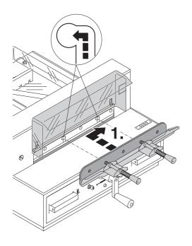
Place the blade to be exchanged, using the blade changing tool, into the blade carrier and push to the top and to the left.(1.) (see picture A) while doing so push both springs back.
