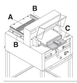
Position the paper on the backgauge (**A**) and side lays left or right (**B**).
