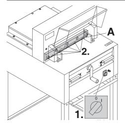
Tighten the blade screws (A) on the right hand side.
