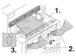
Close the safety guard (1.) Lower the blade by pressing both cutting buttons (2.). Keep one button pressed and turn off the main switch (3.).
