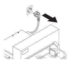
Disconnect from the mains before starting any service work or before removing the panels!
