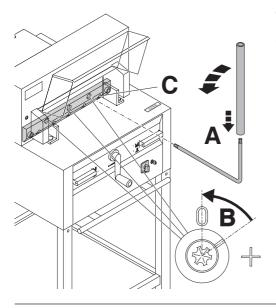
The 3 eccentrics are now exposed and should be turned counter clockwise to position "0" with the special wrench and attachable extension pipe (**A**) (in the tool set). The slot must correspond to position "0" (**B**). Unscrew the blade screws (**C**) on the right hand side.
