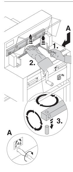
Take out the cutting stick with a small screwdriver. If needed the cutting stick can be turned or exchanged.
