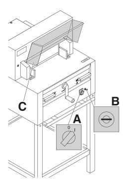
Position the main switch 4 to "I" (**A**). Insert the key 6 for the control system and move it to the right (**B**). Open the safety guard 6 (**C**). The machine is now ready for use.
