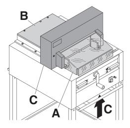
Operating the machine without safety device is forbidden! (Front safety guard (**A**), rear screwed safety guard (**B**) and panel (**C**).
