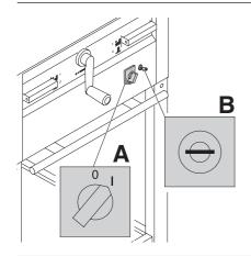
Main switch to position "I"? (A) Control system activated? (B) (Turn key to the right) Check the units fuse and the on-site circuit breaker! Release a cut see page 19 and 20.
