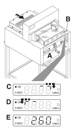
The measurement is set with the backgauge crank.(**A**) The symbol – rotary direction –
