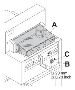
Before working with the machine and after every blade replacement the automatic cut-off function of safety guard ( $\mathbf{A}$ ),(correct if distance between cover and table is < 20 mm) main switch ( $\mathbf{B}$ ) and control panel ( $\mathbf{C}$ ) must be checked.
