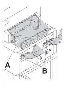
The dangerous cutting movement is safeguarded by a movable guard (**A**) and a safety two-handed control system! (**B**)
