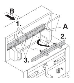
Lightly tighten 2 of the 5 blade screws (1.). Remove the blade changing tool (2.). Lightly tighten the remaining blade screws (3.). Lightly screw in the right blade screw (A) when the blade is lowered.
