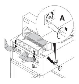
Paper cutting test. If the last sheet or several sheets are not completely cut, gradually turn the knob for blade depth adjustment (A)  $\frac{1}{4}$  turn to the right until the paper is cut along the entire length. Do not set too low as blade will become blunt sooner.
