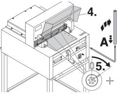
Open the safety guard (4.). With the special wrench (B) the 3 eccentrics should be screwed down (5.) until the paper is cut along the entire length of the blade (The blade must remain parallel, not too deep into cutting stick).
