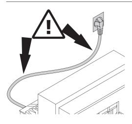
Protect mains cable against heat, oil and sharp edges!
