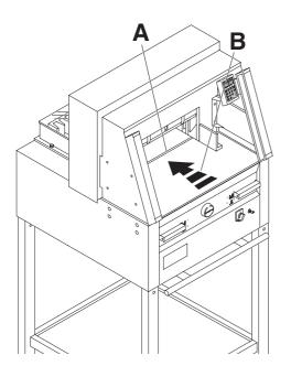
Optical cutting line (**A**) that indicates the exact position of the cut. Blade cuts on the front edge (**B**) of the light beam. (Only use when no exact cut is required).
