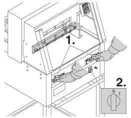
Lower the blade by pressing both cutting actuators (1.). Keep one actuator pressed and turn off the main switch (2.).
