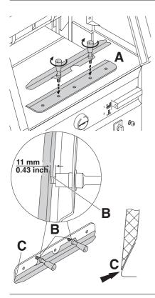
Take the exchange blade carefully out of the blade box and screw it to the blade changing tool (A).
