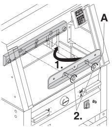
Place the blade to be exchanged with the blade changing tool (**A**) mounted (**1**.), into the blade carrier and push it up to the top and screw it into place with the grips (**2**.).
