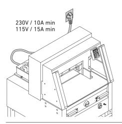
Connect the power cord to a single phase socket.
