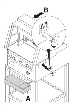
Turn the blade depth adjustment screw to the left until it stops. (Screwdriver found in tool set (A)) or tool holder (B).
