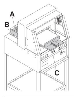
Position the paper on the backgauge (**A**) and side lays left or right (**B**).
