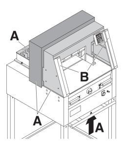
All components which could endanger the operator are covered by a guard!
