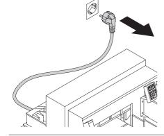
Replacement of blade and cutting stick may be performed only when the main switch is switched off!
