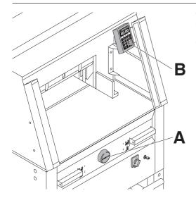
The measurement is set either with the handwheel (**A**) or by programming (**B**) the cutting measurements. Measurement is shown on the display in inches or cm (**B**).
