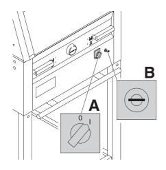
Main switch to position "I"? (A) Control system activated? (B) (Turn key to the right) Release a cut see page 21.
