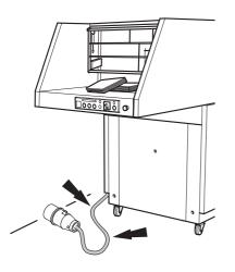
Protect mains cable against heat, oil and from sharp edges.
